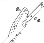
4 Unfold the handlebar and fasten the knob on both sides of the machine. Adjust to a suitable height. For more information, see "Adjustment". 5 Place the wires in the cable bracket. Make sure the wires are not twisted around each other. Fasten the cable bracket underneath the handlebar.
