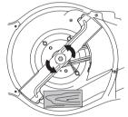
Make sure the blade bracket is free of damage. Also check that the cutter bolt is undamaged and that the engine shaft is not bent.
